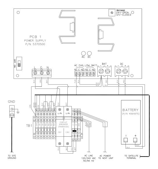
Figure 1-1 – FTW 175-SAT Internal Wiring and Component Layout
