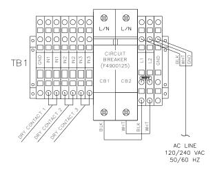
Figure 3-1 – Terminal Block TB1 Layout, Dry Contact Wiring, and AC Termination
