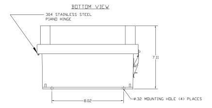
Figure 3-4 – Enclosure Mounting Footprint
